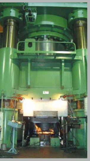
Our 9,000 tonne hydraulic forging press
