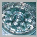
After third stage forging, the wheel is ready for machining
